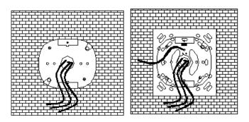
Step 4:Finish wiring, Put all wires inside light holder. Then fixed the lamp by screwing the left and right sides of the lamp holder.
