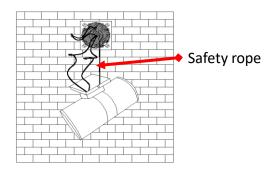
Step 5: Use waterproof silicon seal the gap between lamp and wall if it is ,double protection for using in outdoor.
