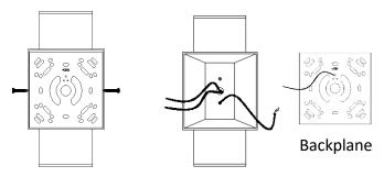
Step 3:Hang the safety rope on the backplane, the light is hanging and hands are free for wiring. Then wiring with the wiring cap.
